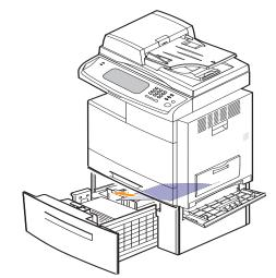
If the jammed paper is not visible, or if the paper is stuck, stop pulling and continue on to step 5.
